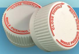
Involves transferring a colored ink to an embossed cap by printing rollers. Requires a raised logo created by a mold insert to make an embossment, which is 'rolled over' through an offset printing machine.
