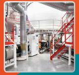
Blown film: Complete lines for co-extruded film up to 11 layers and products up to 82 feet (25 meters) in circumference for food packaging, construction, agricultural, industrial and bags for heavy-duty applications.
